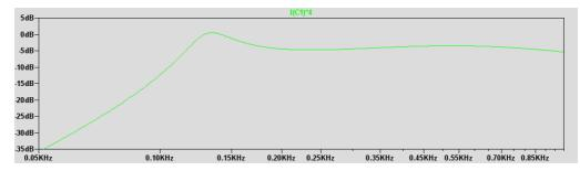
You can see that the response peak has moved LOWER in frequency, which is certainly unexpected, but more significantly, the response doesn't drop 3 dB at 250 Hz, because the impedance of the loudspeaker is rising as the frequency goes down. It doesn't drop away until the frequency is below the response peak, where it plunges twice as rapidly as it does in the absence of the capacitor.
