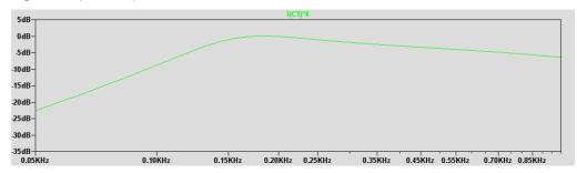
When we add the 100  $\mu$ F in series, the frequency response of the modelled loudspeaker does this. It waves about a bit above 200 Hz as the capacitor and voice-coil inductance have their own private battle:
