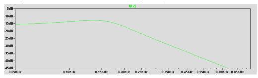
where the dB scale is purely relative. Adding the capacitor doesn't do what we expected:
