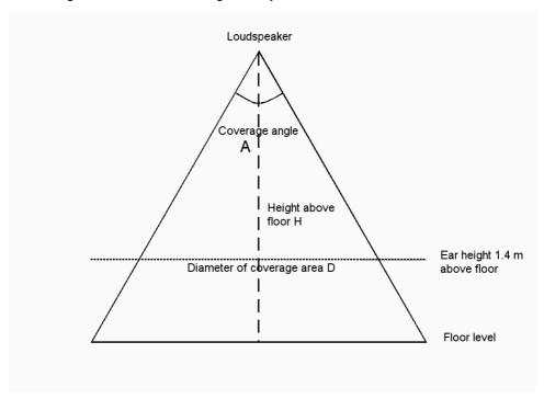
The diameter of the coverage area (a circle if the loudspeaker does not have a non-coaxial tweeter) can be calculated either by Pythagoras or trigonometry (two sides of the same coin). Using trig, we get:
