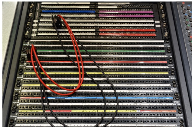
1. A typical central audio signal patch in a recording studio with over a thousand signal lines and millions of possible valid permutations of interconnect. All grounds are connected at all ends of the audio lines (including here) to provide quiet critical operation.
